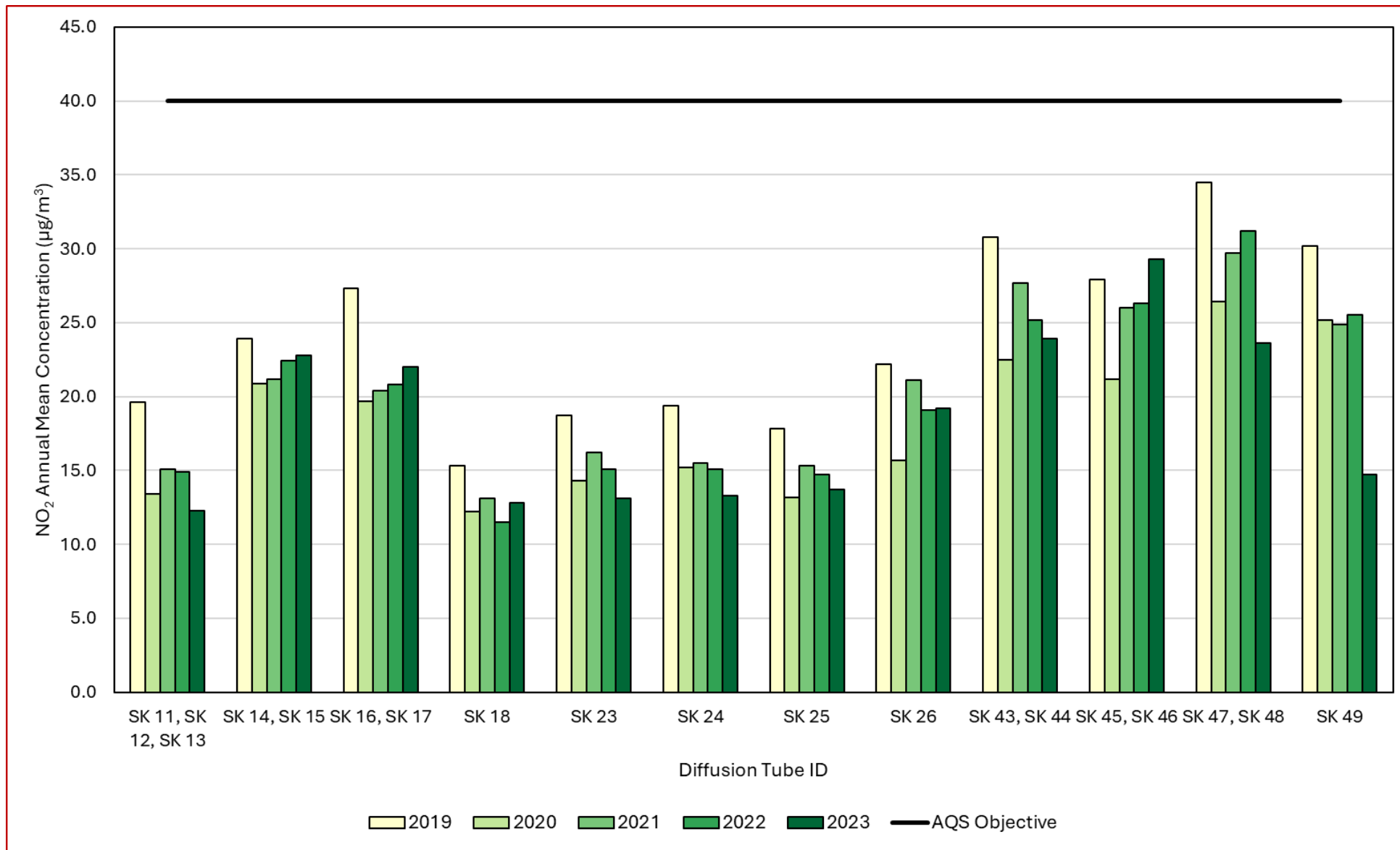
Figure A.3 – Trends in Annual Mean NO 2 – Diffusion Tubes (Sites in Grantham (Outside AQMA))
