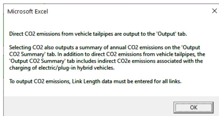
The CO<sub>2</sub> output creates an **Output CO<sub>2</sub> Summary** sheet inclusive of direct CO<sub>2</sub> emissions from tailpipe and indirect CO<sub>2</sub>e emissions associated with the charging of the batteries of electric and plug-in hybrid cars and LGVs, in tonnes/annum.
